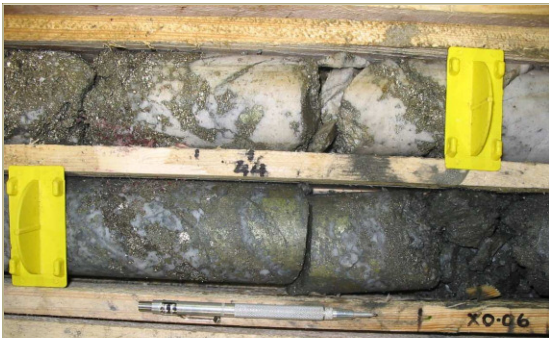
Figure 10-3: Quartz-Sulphide Vein in Drill Core
