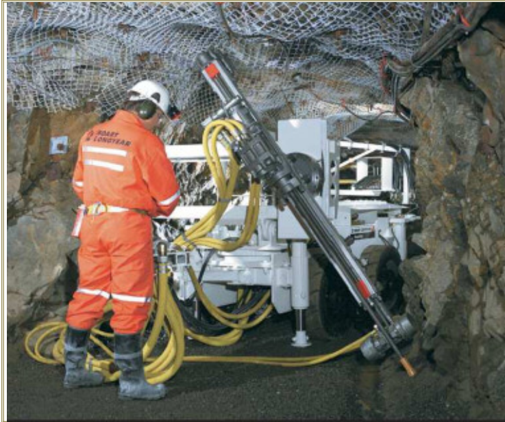
Figure 16-5: Production Drilling in Narrow Vein
