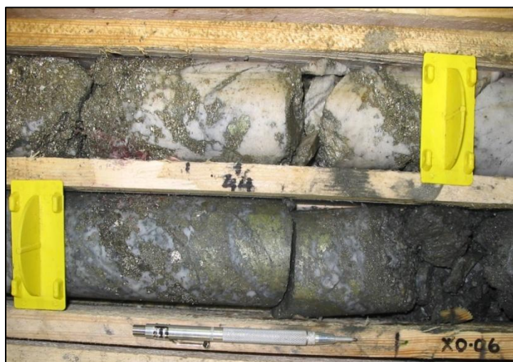
Figure 10.3 Quartz-Sulphide Vein in Drill Core
