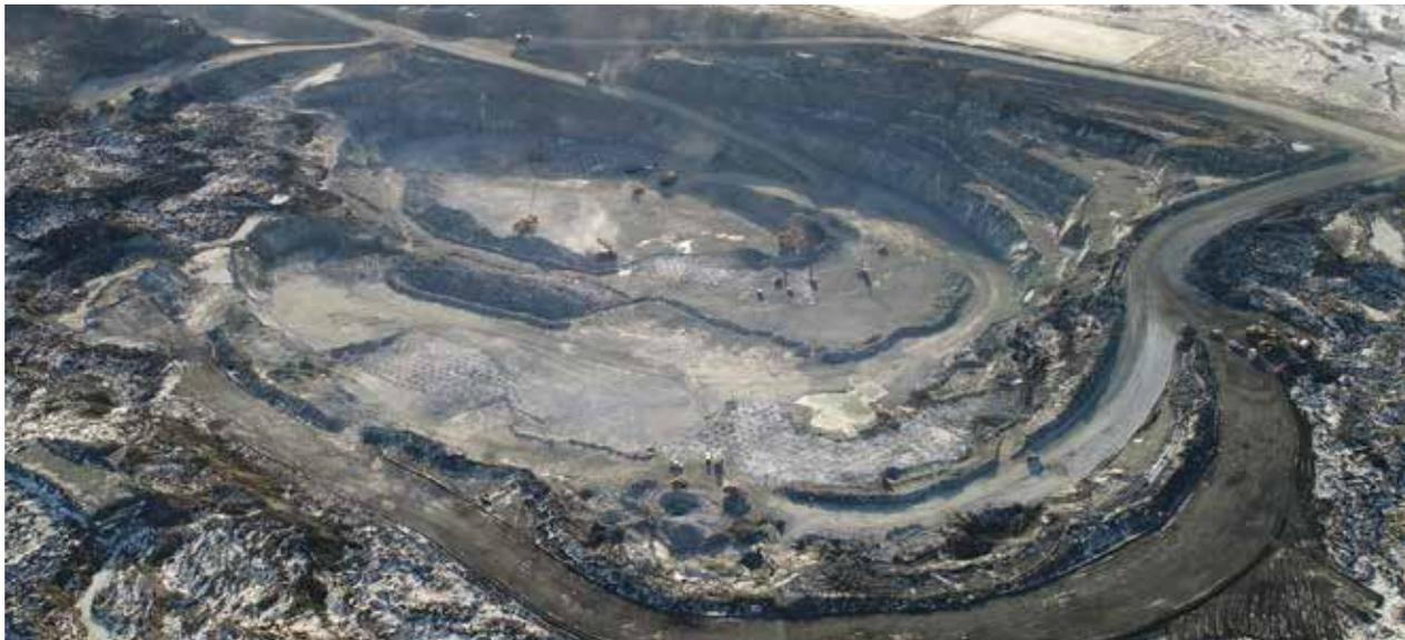
*Aerial view of the open pit; from surface to the pit floor is currently 80m*
