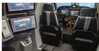
King Air 350i Full Flight Simulator
