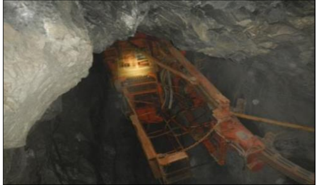
Alimak raise climbing equipment begins climbing up the first raise
