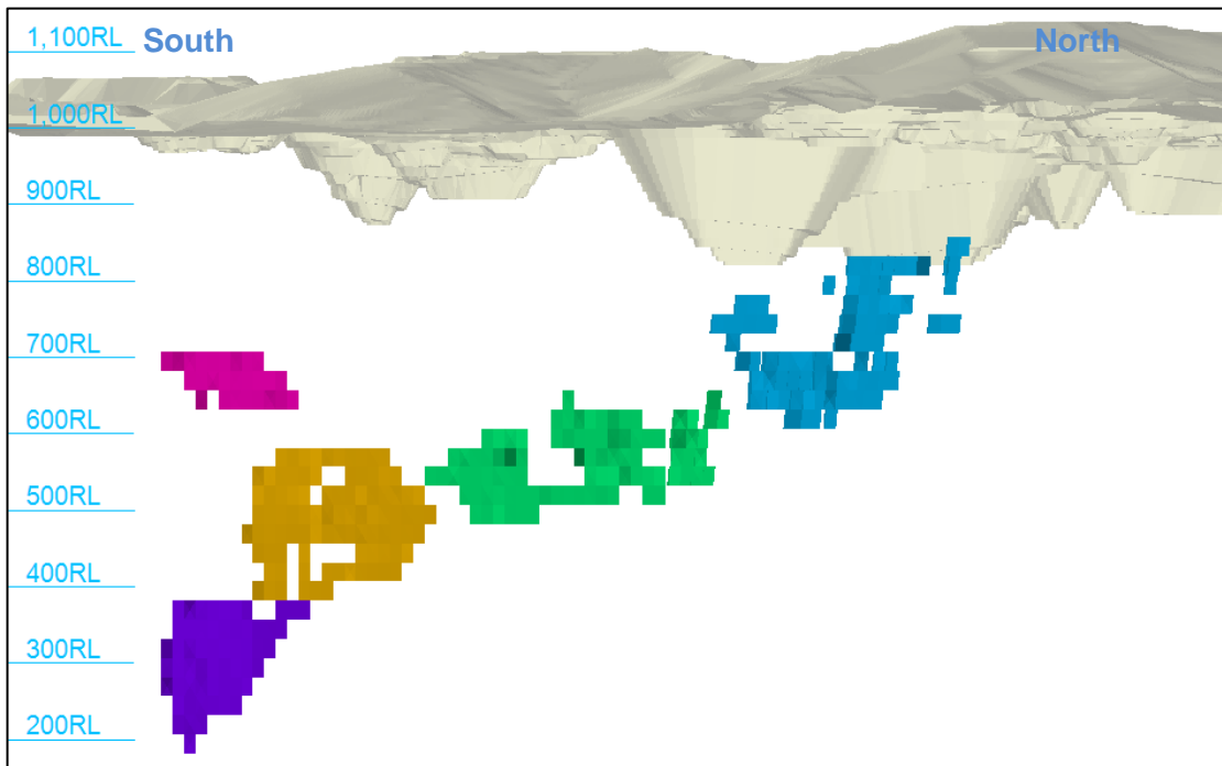
Figure 15-11: View looking west of stopes included in Wassa Underground mine plan
