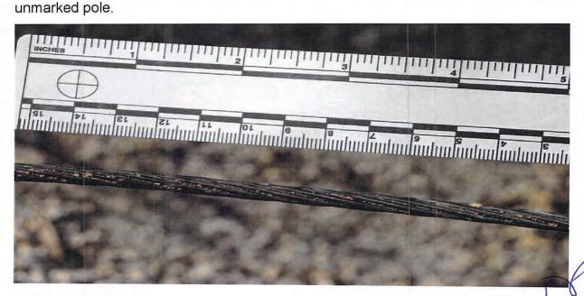
Conductor #2 (middle conductor) Approximately 12 inches of conductor was removed and packaged as E-10. This section of conductor was located approximately 32 feet uphill from the insulator on the unmarked pole. This section of conductor showed signs of fresh arcing and beading in multiple spots over the approximate 12-inch section.
