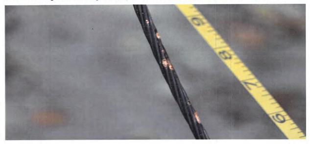
Conductor #3 (north conductor) Approximately 4 feet of conductor was removed and packaged as E-9. This section of conductor showed signs of tree bark and material transfer from approximately 34 feet uphill of the unmarked pole to within approximately 12 inches of the insulator on the unmarked pole. It also showed black remnants where the tree trunk made constant contact after coming to rest. This area was located approximately 33 inches uphill from the insulator.
